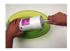
DO NOT pour any of the wastewater down the drain since it may contain substantial amount of mercury. The black vinyl cap then have to be placed again over the inflow hose barb in order to seal this side of the filter. The filter is then angled at 45 degrees so that the outflow barb is pointed up and the process is repeated. The black vinyl cap then securely placed on the outflow hose barb.
