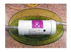
3 \_ The inflow side of the filter is angled up approximately 45 degrees and vacuum hose is pulled off the inflow side hose barb. The end of the vacuum lines should be kept in the tray to trap any wastewater that may remain in the lines. Any wastewater that collects in the tray should be disposed of appropriately.
