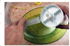
4 \_ Photograph showing the used filter disconnected from the vacuum lines. The black vinyl caps are securely placed on both ends and the used filter is ready for recycling. A new DDS2011 amalgam separator can now be installed by placing the vacuum hoses on the appropriate hose on the appropriate hose barb fitting.
